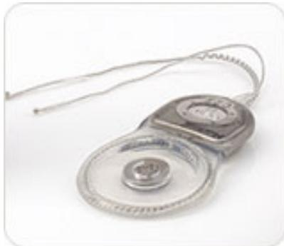
These are the parts of the device implanted by the surgeon during the cochlear implant operation. They include the internal receiver/ stimulator package (with the internal magnet). It lies under the skin behind the ear, and can be felt if touched gently.
